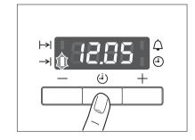
2. Using the + or — button set the desired switch-off time.
